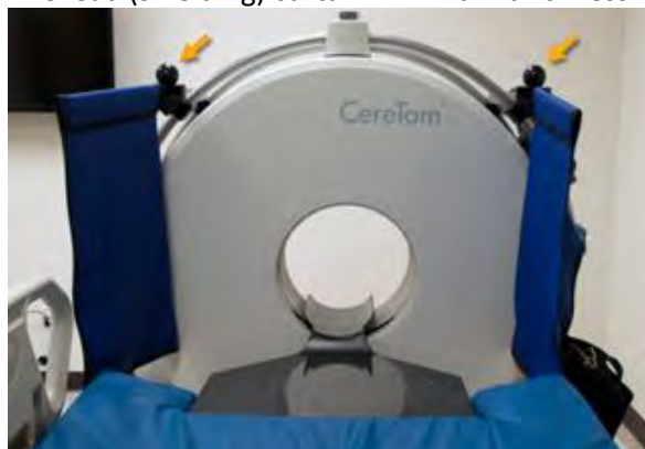
Figure 56: Shielding curtains positioned with knobs
