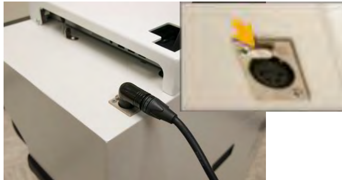
Figure 432: SDS joystick cable connected to SDS, arrow pointing to release button
