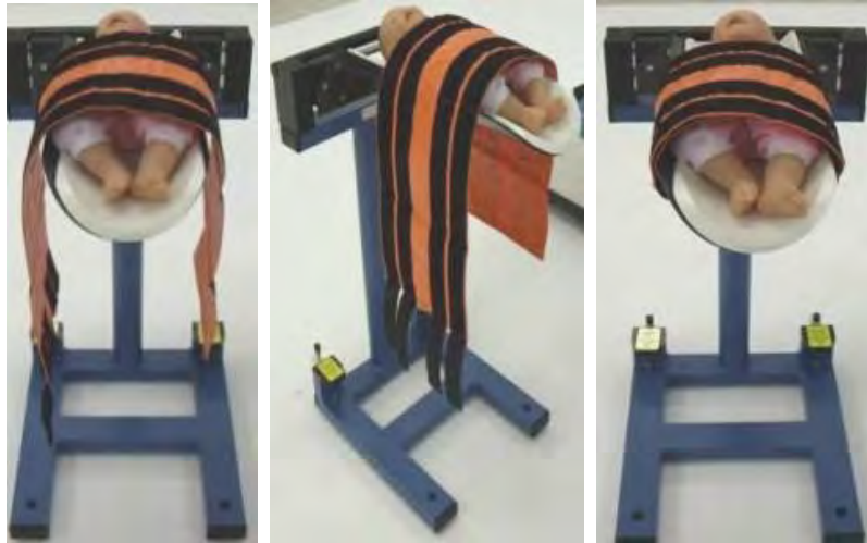
Figure 417: Applying pediatric strap onto the platform (three views)
