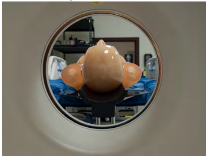
Figure 52: Ensuring placement of patient's neck directly under rotating laser light
