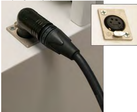
Figure 437: Joystick connector (attached and unattached)
