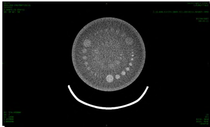
Figure 223: Catphan 515 using 120kV, 7mA, 6 secs, and 5mm slice
