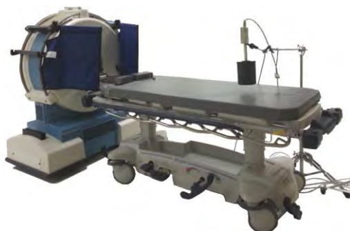
Figure 234: System setup for scatter measurements
