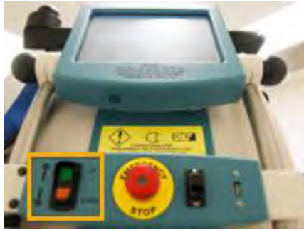
Figure 44: Rocker-Switch-Lift Up and Down buttons
