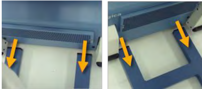
Figure 419: Scanner shown to (easily) slide over platform base (two views)
