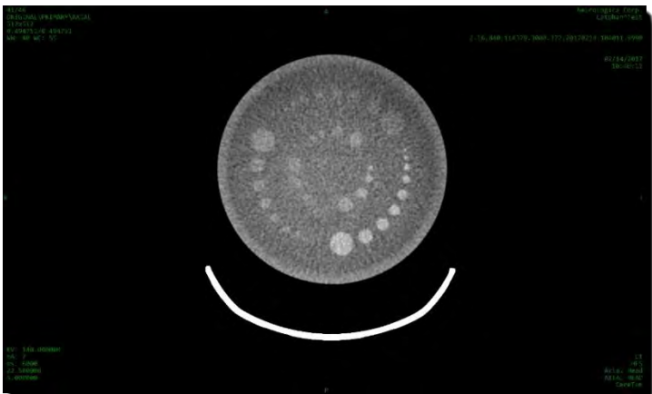
Figure 224: Catphan 515 scanned using 140kV, 7mA, 6 secs and 5mm slice
