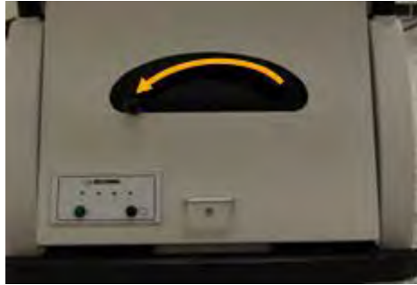
Figure 434: Locking lever in unlocked position
