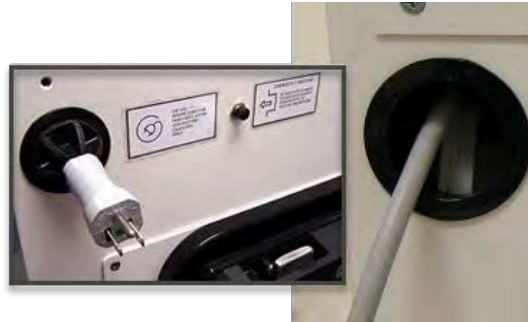
Figure 430: SDS retractable power cord –retracted (left) and not retracted (right)
