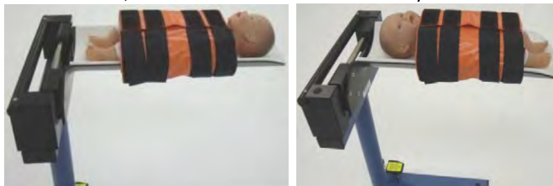
Figure 418: Proper position of neonate/infant for head scans (left) and body scans (right)
