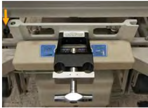
Figure 397: Bed adapter without posts insertion (setscrew showing under arrow)
