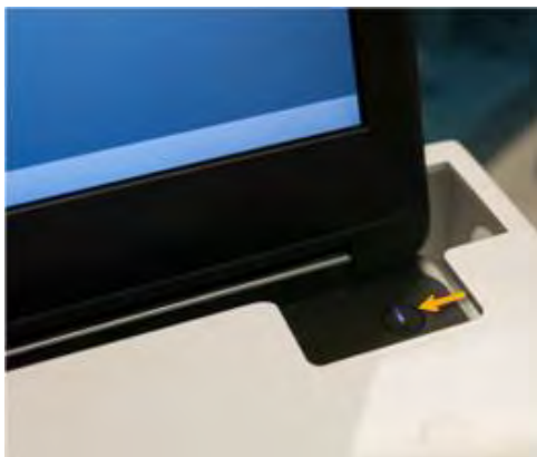
Figure 57: Workstation's Power on button (in this illustration, workstation mounted in SDS)
