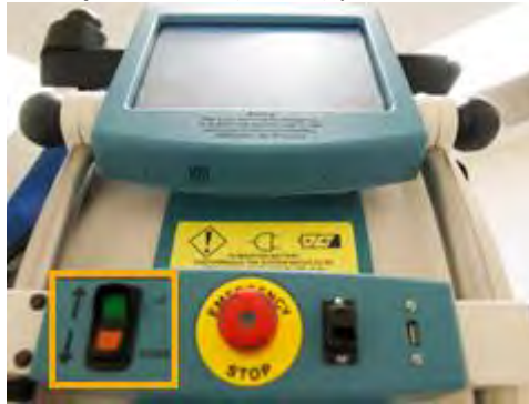
Figure 435: Rocker-Switch-Lift Up and Down buttons
