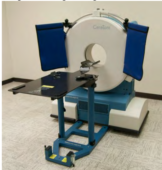
Figure 413: Pediatric platform positioned by the scanner
