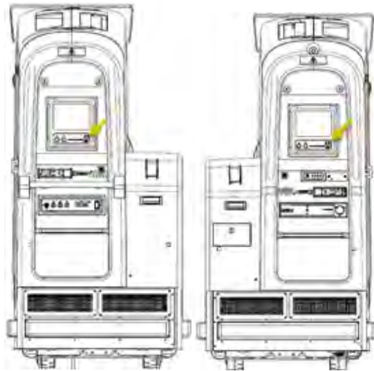
Figure 7: BodyTom Elite E-STOP locations (right and left)
