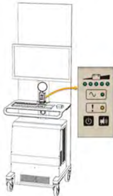
Figure 40: Workstation remote power display
