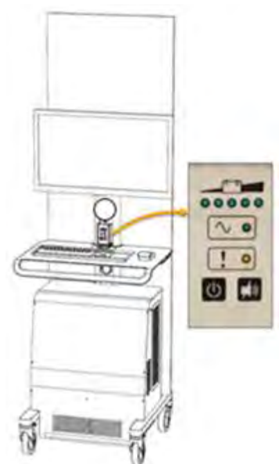
Figure 39: Workstation remote power display
