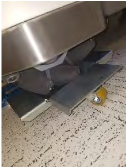
Figure 300: Correct placement of Omniwheel on dolly
