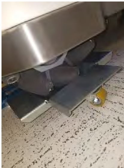
Figure 295: Correct placement of Omniwheel on dolly
