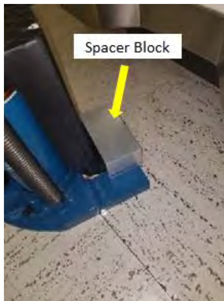
Figure 290: Placement of space block
