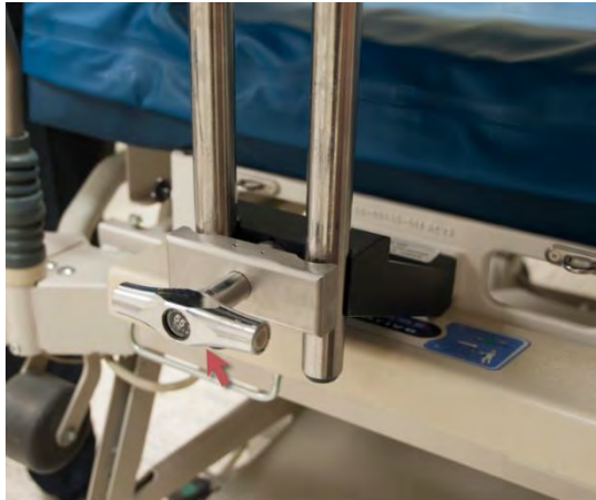
Figure 32: Bed adapter with T-square
