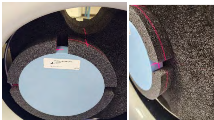
Figure 130: Set the laser in the middle of solid water portion of the phantom
