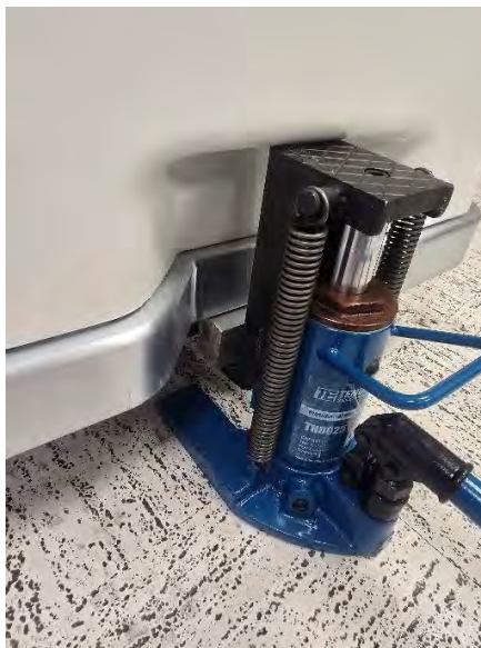
Figure 286: Proper placement of Jack
