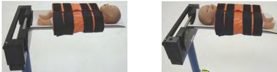
Figure 275: Proper position of neonate/infant for head scans (left) and body scans (right)
