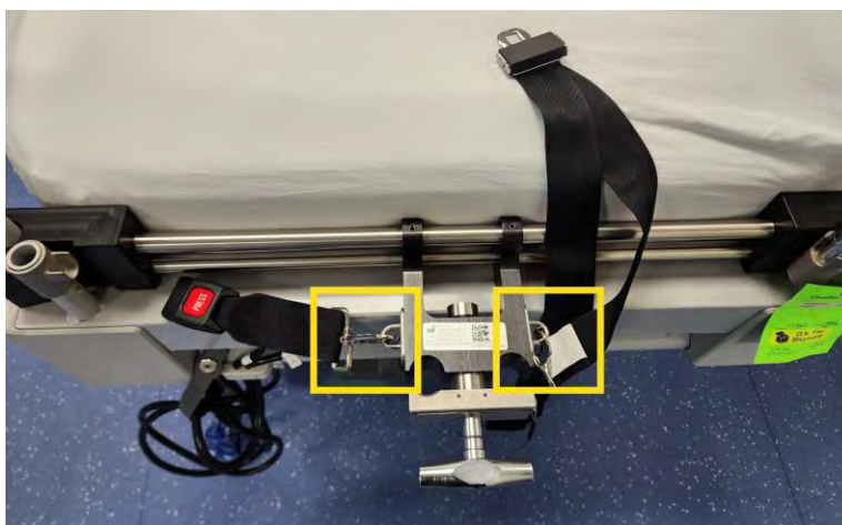
Figure 254: Straps attached to bed adapter
