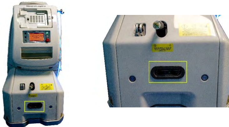
Figure 22: Optional drive view camera
