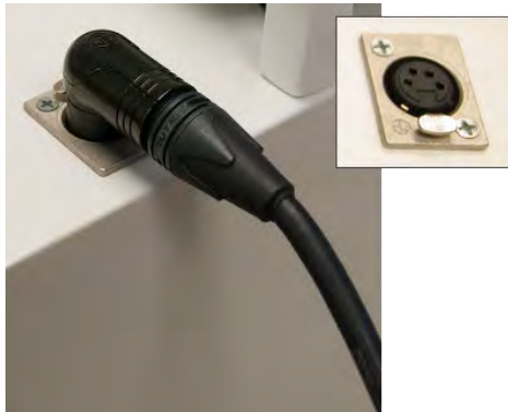
Figure 421: Joystick connector (attached and unattached)
