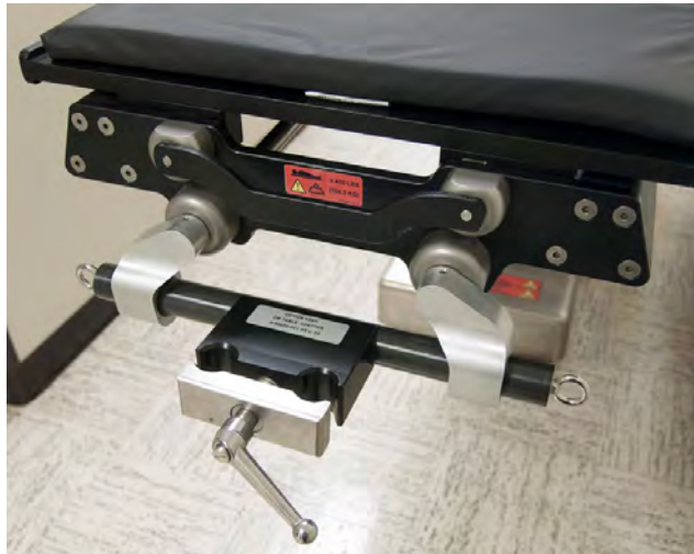
Figure 397: OR table adapter attached to mount
