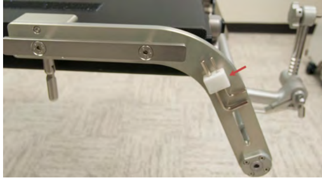
Figure 399: Doro park-bench adjustment using Allen wrench
