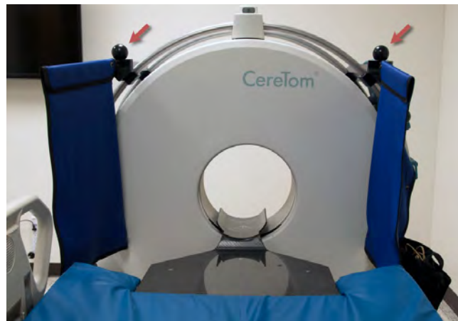
Figure 49: Shielding curtains positioned with knobs
