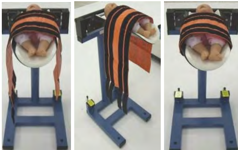
Figure 390: Applying pediatric strap onto the platform (three views)
