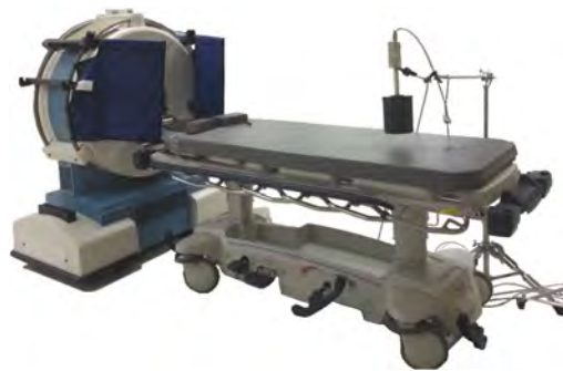
Figure 220: System setup for scatter measurements
