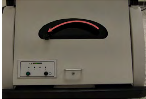
Figure 418: Locking lever in unlocked position
