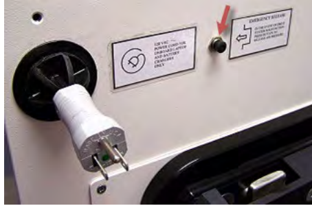
Figure 415: SDS pneumatic emergency release
