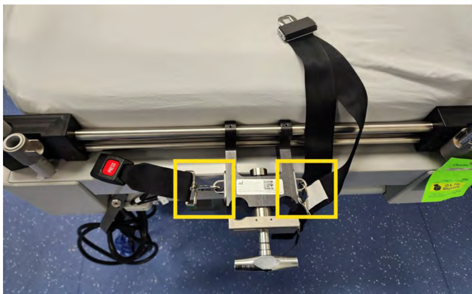
Figure 364: Straps attached to bed adapter
