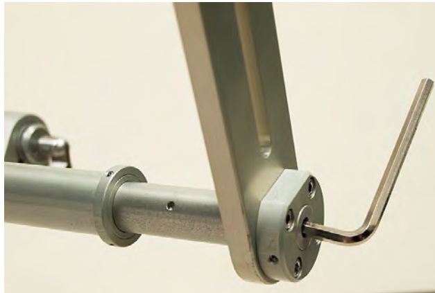
Figure 400: Doro bench adjustment with Allen wrench
