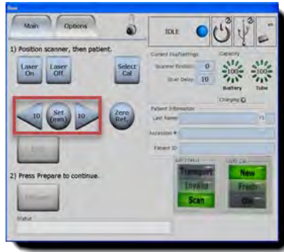
Figure 40: Active Left and Right buttons, and Set (mm) button
