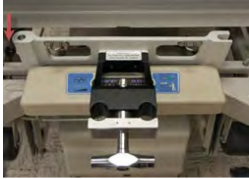
Figure 367: Bed adapter without posts insertion (setscrew showing under arrow)
