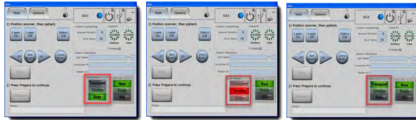
Figure 37: Lift Status: Scan, Invalid, and Transport modes
