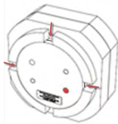
Figure 196: Phantom's etchings appear on top and sides
