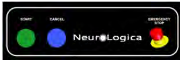
Figure 7: Close-up of the scanner control panel and the E-STOP button
