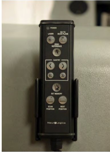
Figure 15: BodyTom 64 remote-control pendant
