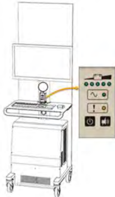
Figure 39: Workstation remote power display
