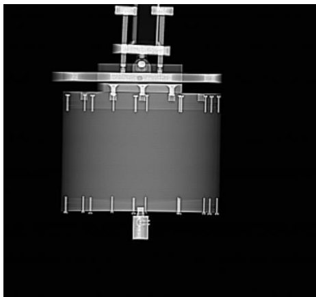
Figure 3: the AP scout of a 20 cm water phantom and the estimated radius based on the scout.
