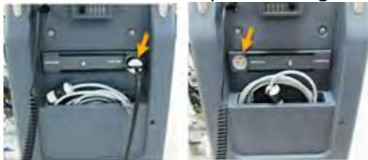
Figure 23: AC cord and storage on scanner (120V left plug in or 240V right plug out)
