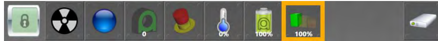
Figure 201: Air freshness icon changes as the air quality drops from green to yellow to red
