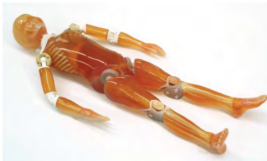
Figure 159: The pediatric body phantom
