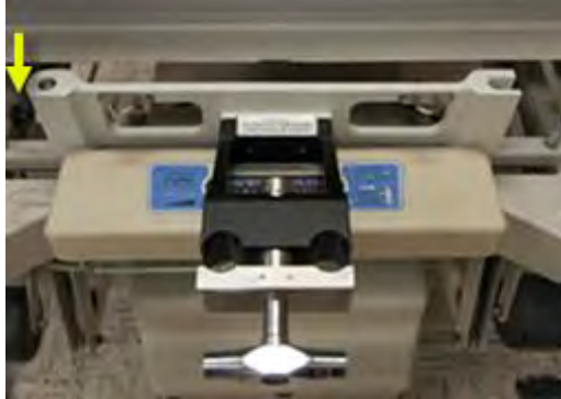
Figure 251: Bed adapter without posts insertion (setscrew showing under arrow)
