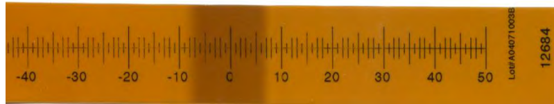
Figure 153: The measured beam width of the OmniTom Elite scanner
