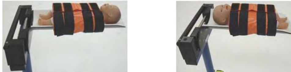
Figure 268: Proper position of neonate/infant for head scans (left) and body scans (right)
