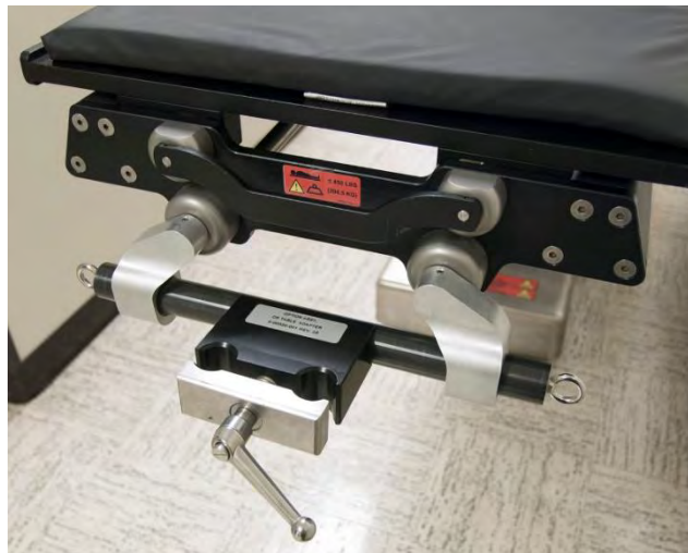
Figure 273: OR table adapter attached to mount
