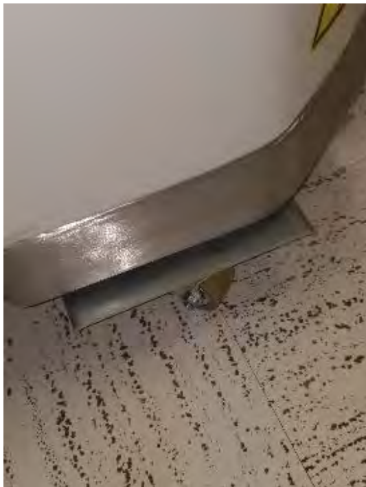
Figure 287: Proper placement of dolly
