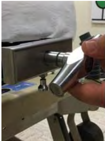
Figure 256: Correct install depth
