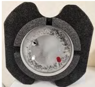
Figure 138: OmniTom with PCD QA Phantom
