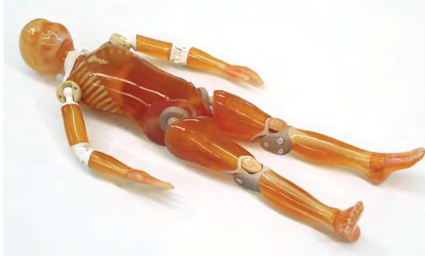
Figure 153: The pediatric body phantom
