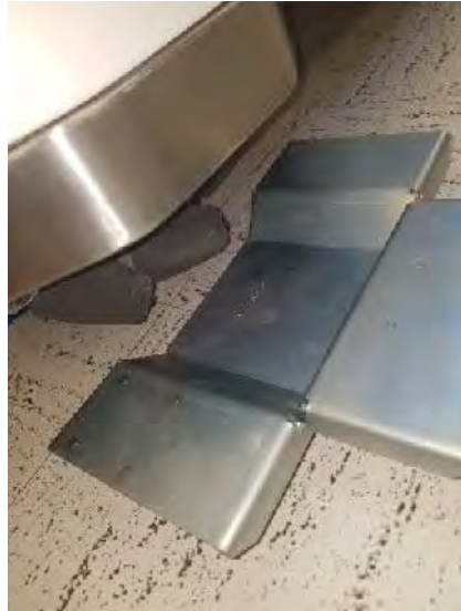
Figure 287: Move the dollies into place
