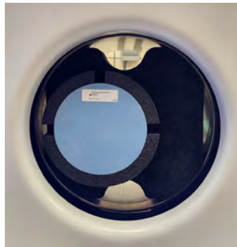
Figure 129: Water phantom inserted in the scanner bore
